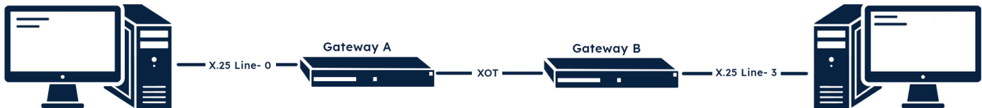
Example configuration showing an X.25 lines at each end with the network running XOT (X.25 over TCP/IP)
