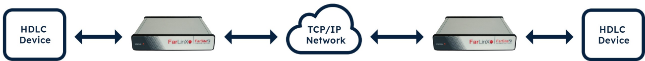
Diagram illustrates an HDLC connection being bridged over the TCP/IP network such as the Internet using a FarLinX Connect Mini at each end
