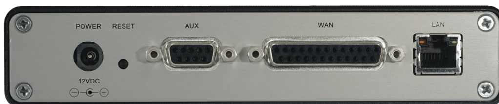
Rear panel view showing, 12V, 1.5A power input, system reset button, AUX port (not used), WAN port for the HDLC connection and a LAN connection
